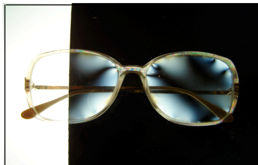
Figure 14. These eyeglasses are resting on a light box covered with a sheet of polarizing film. A second piece of film oriented at right angles to the first is covering the eyeglasses on the right. Stress in the glass lenses is apparent under the top polarizer.
